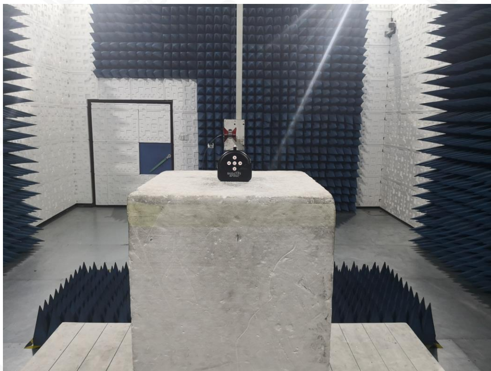
FCC RADIATED EMISSION TEST SETUP ABOVE 1GHZ
