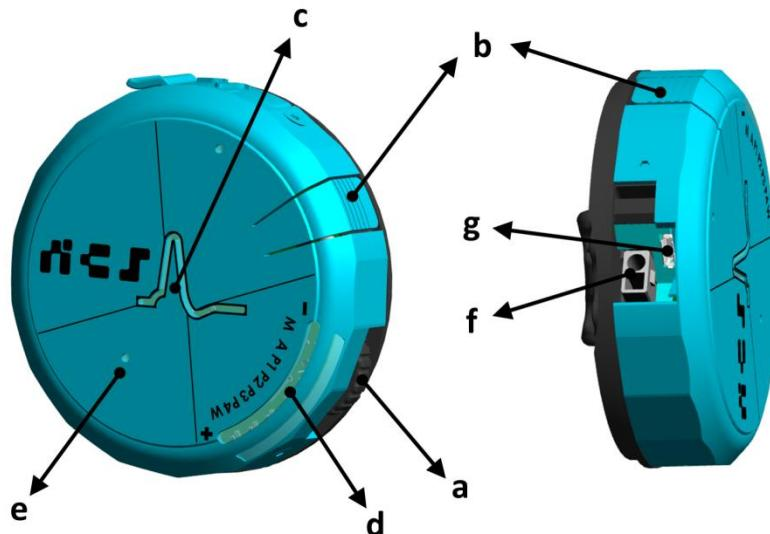
The device is managed by rotating the wheel (a) and pressing the button (b). The status of the device (on, off, stimulation, charging) is indicated by the yellow led in the center of the device (c). The management of the menu and the regulation of the intensity of the stimulation are revealed by the turning on, off or flashing of the band of the red leds (d), that are switched on in sequence according to wheel rotation.
