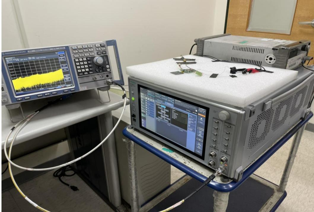
**AC power line Conducted Emission Set up Photo**
