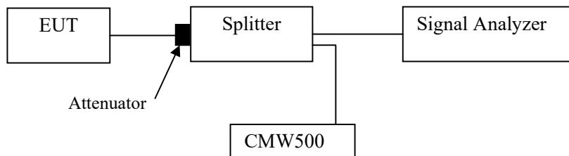
**Transmitter unwanted emissions-at antenna terminals**
