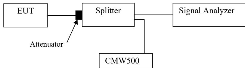
Note: the worst path loss (cable loss and splitter inset loss) among the test frequency range was added into plots.
