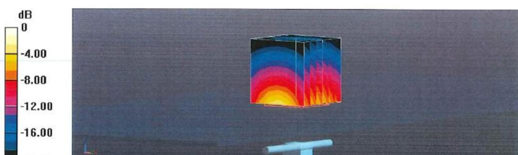
**Impedance Measurement Plot for Head TSL**
