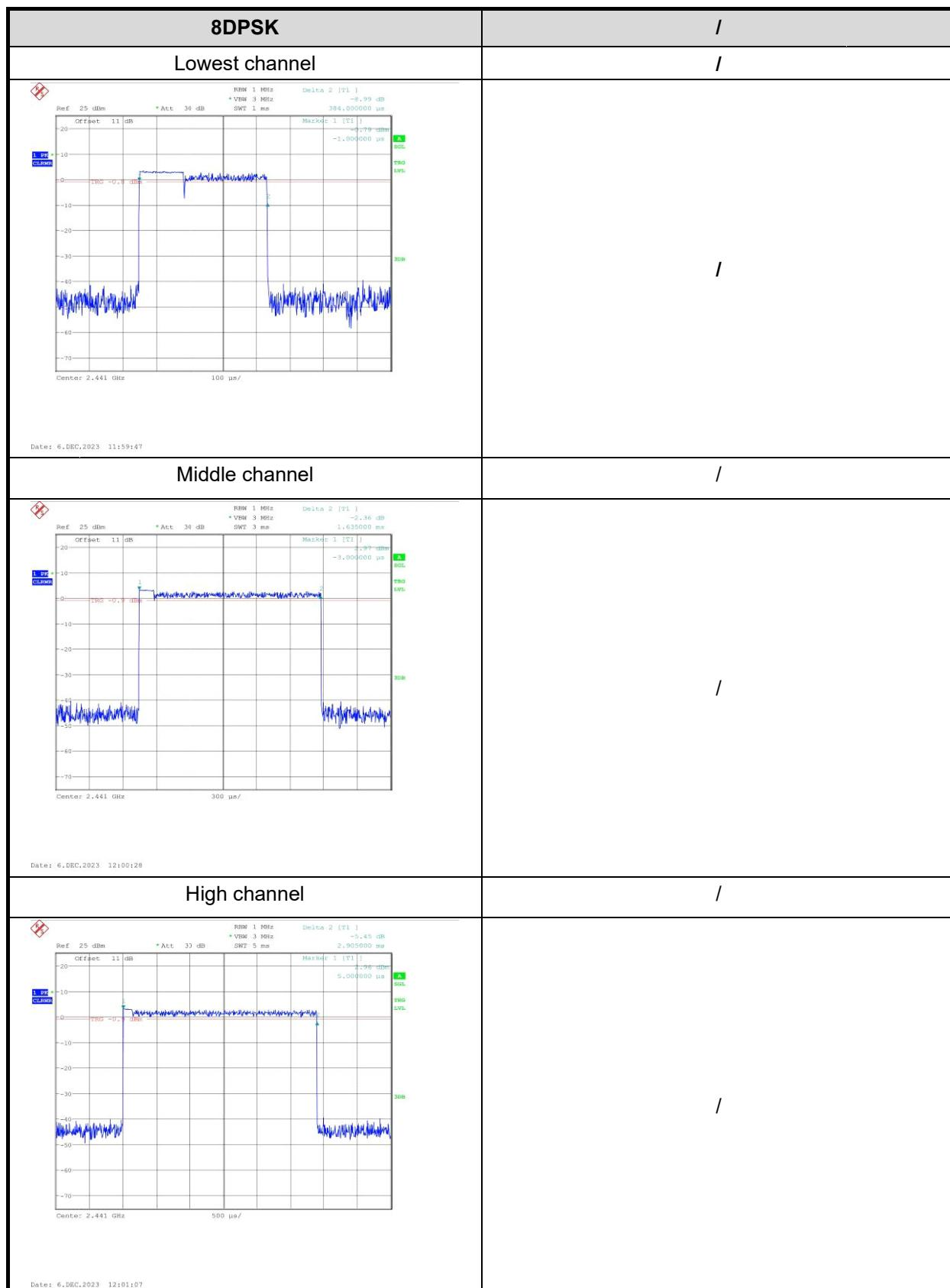
**100kHz Bandwidth of Frequency Band Edge:**
