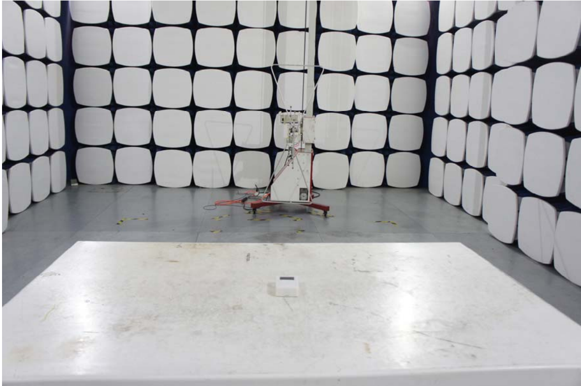
Radiated Setup photo (Below 1G)
