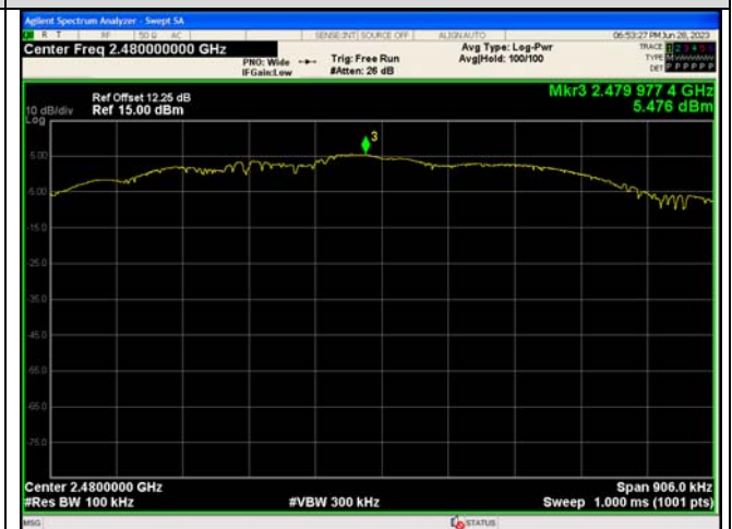
In-Band Reference Level LE_Channel 39
