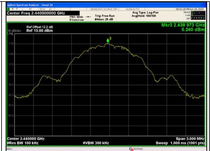
In-Band Reference Level LE_Channel 19
