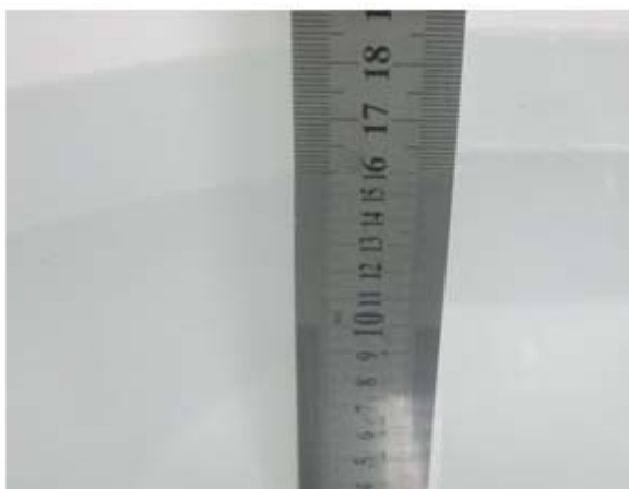
Liquid Height for Body SAR
