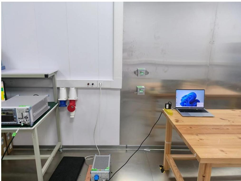
**Radiated Emissions Test Photos****30 MHz to 1 GHz**
