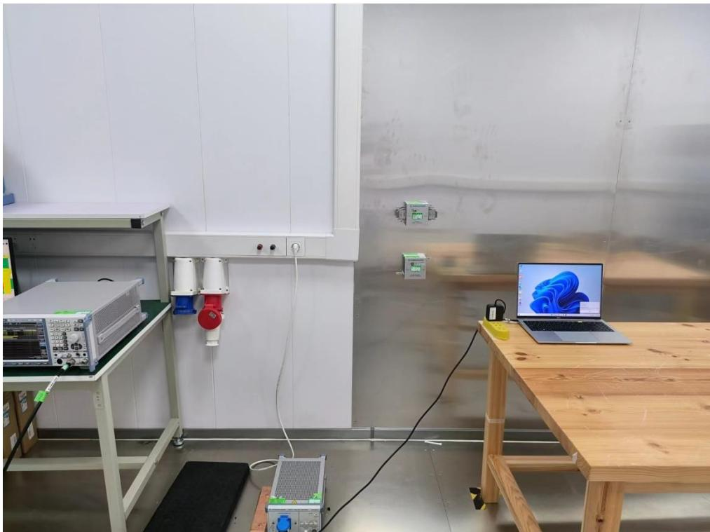
**Radiated Emissions Test Photos****30 MHz to 1 GHz**
