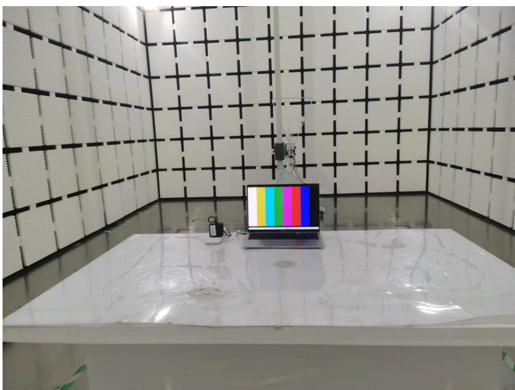
**Radiated Emissions Test Photos****Above 1 GHz**
