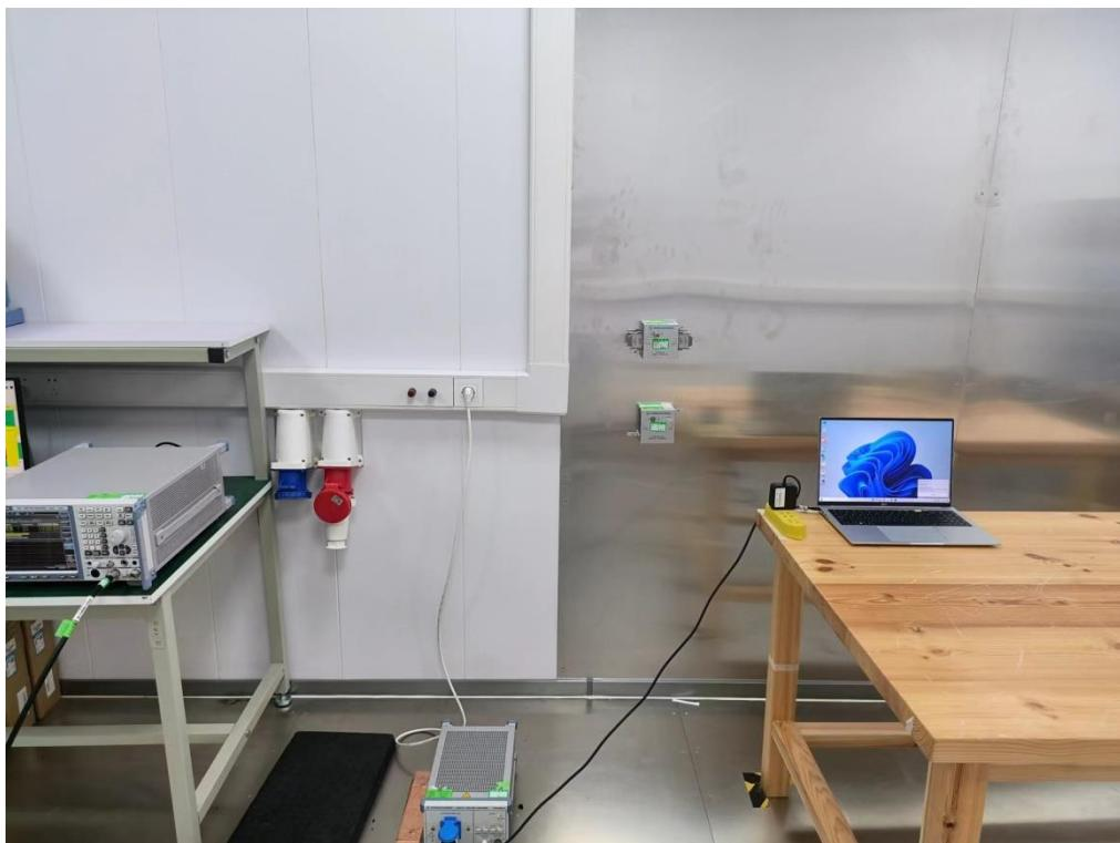
**Radiated Emissions Test Photos****30 MHz to 1 GHz**
