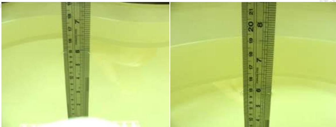
Photo of Liquid Height for Head SAR
