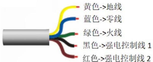
黄色-地线 Yellow - ground wire      蓝色-零线 Blue - null line      绿色-火线 Green - firewire
