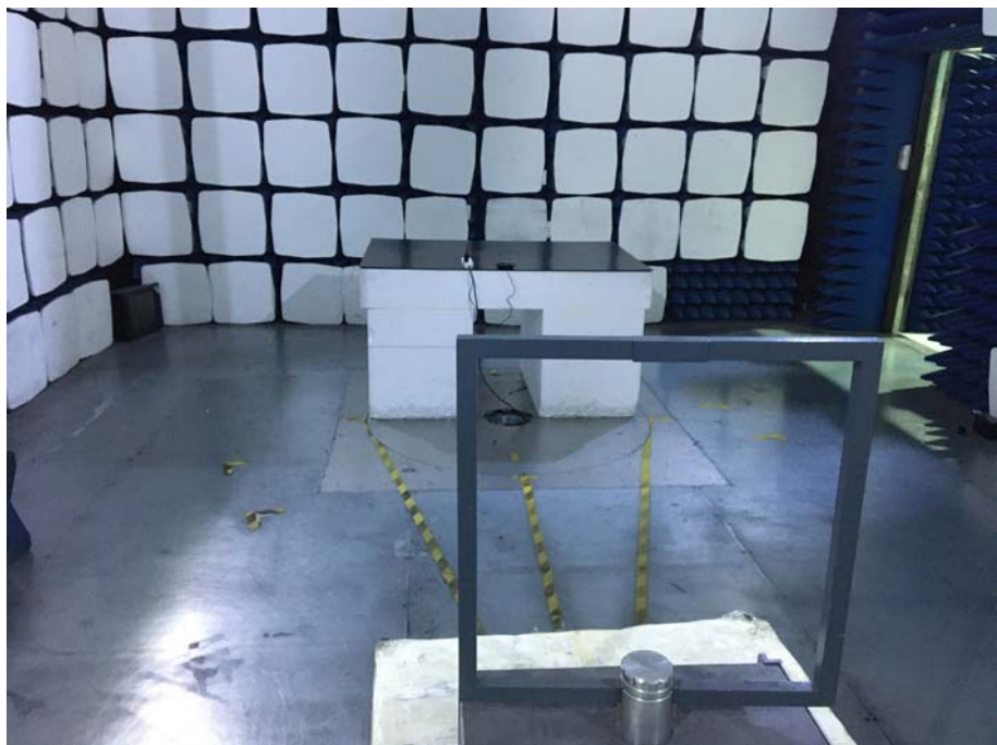
Radiation Emission Test Setup (Below 30MHz)
