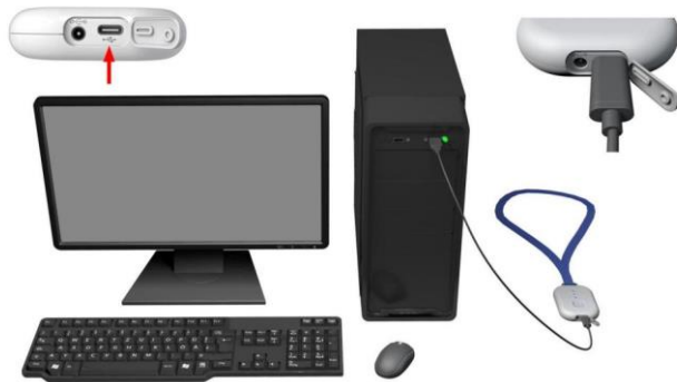
Figure 3-3 Connecting the Data Recorder to a Computer
