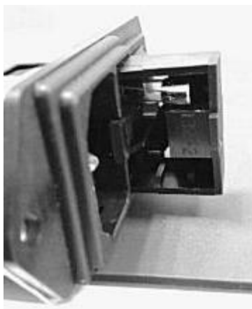
Figure 9- 1: Schematic Diagram of fuse replacement
