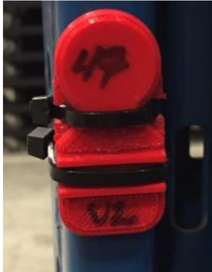
Sample Tag mounted with dual, 4.6mm wide cable ties
