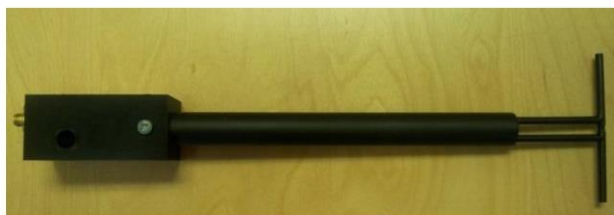
Figure 1 – MVG COMOSAR Validation Dipole
