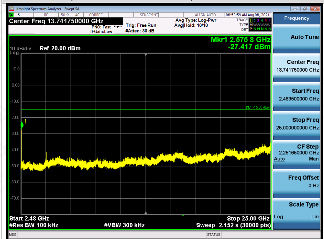
Test_Graph_802.11b_ANT1_2412_1Mbps_Higher Band Emissions
