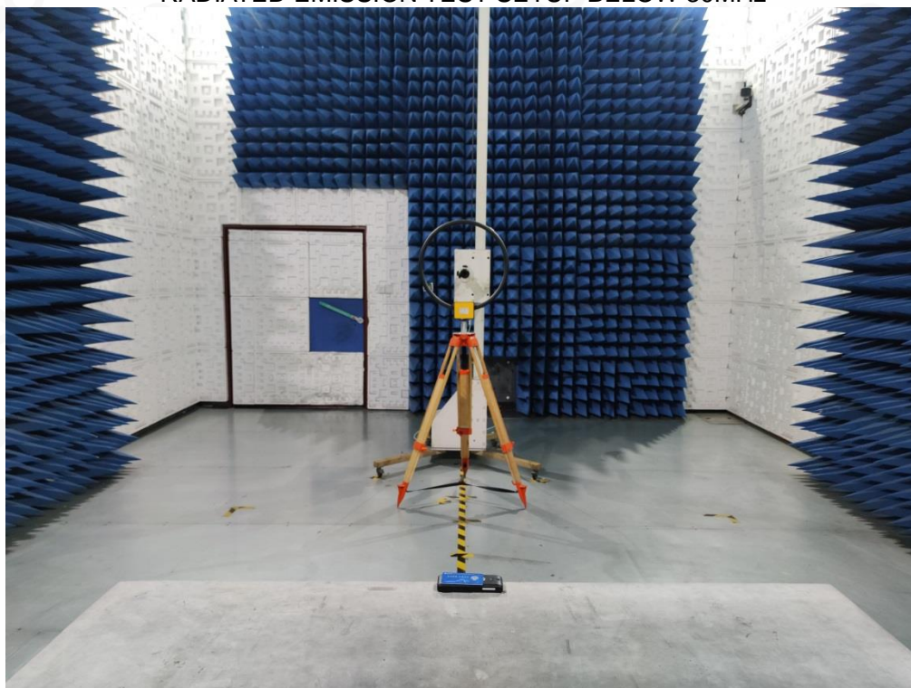
RADIATED EMISSION TEST SETUP BELOW 30MHz
