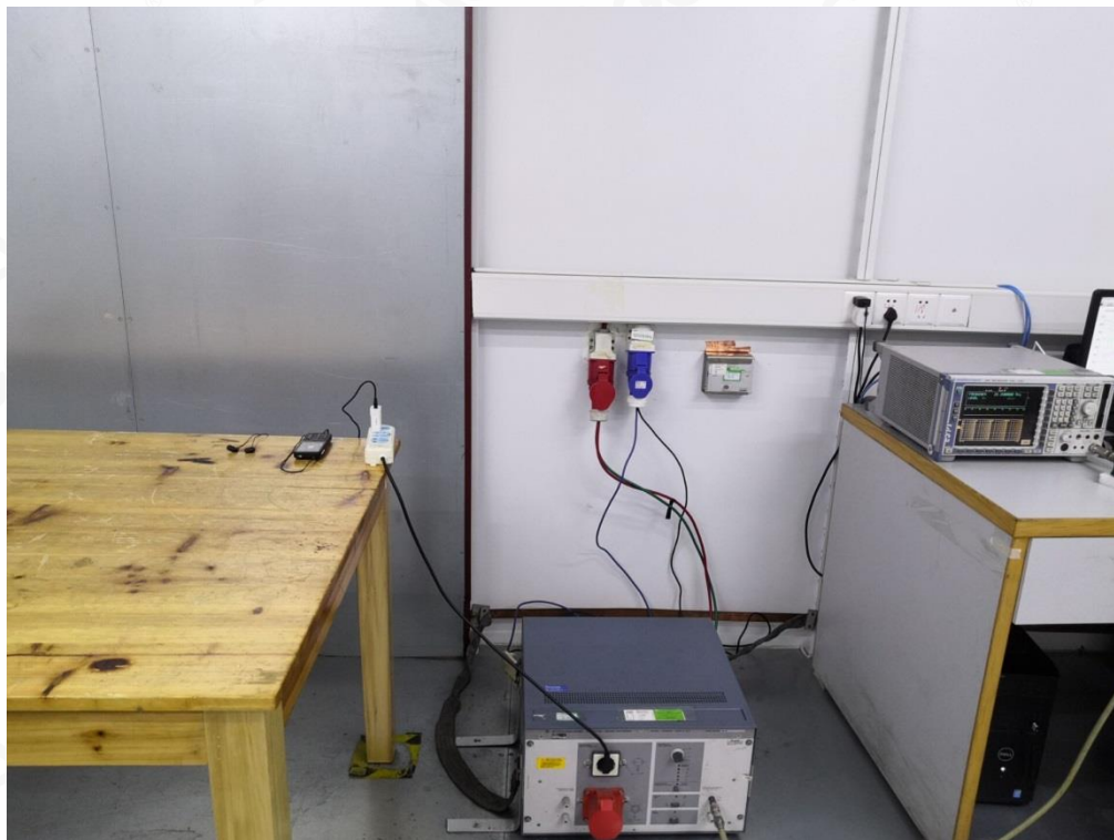
RADIATED EMISSION TEST SETUP BELOW 30MHz
