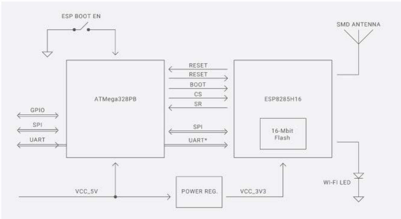
The picture above shows the functional block diagram of the Jolly module.
