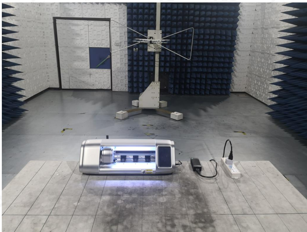
FCC RADIATED EMISSION TEST SETUP ABOVE 1GHZ
