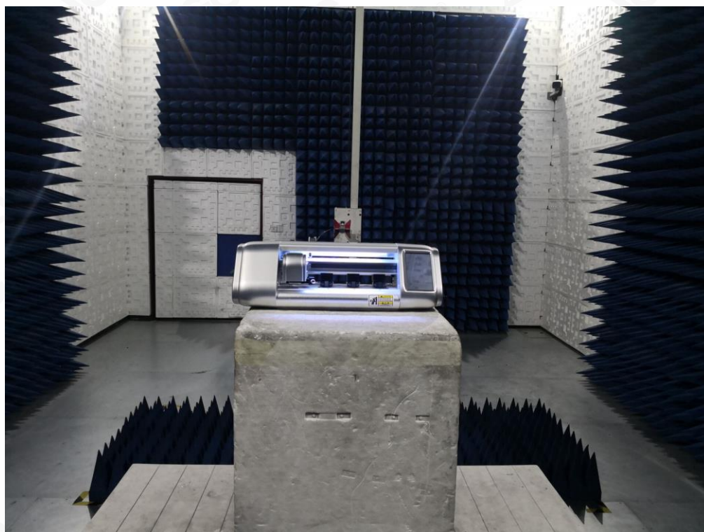
FCC RADIATED EMISSION TEST SETUP ABOVE 1GHZ
