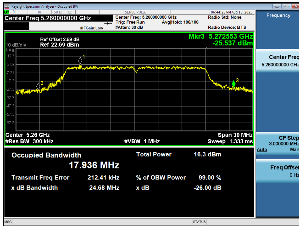
-26dB Bandwidth NVNT ac20 5260MHz Ant1
