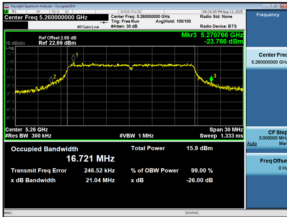
-26dB Bandwidth NVNT a 5260MHz Ant1
