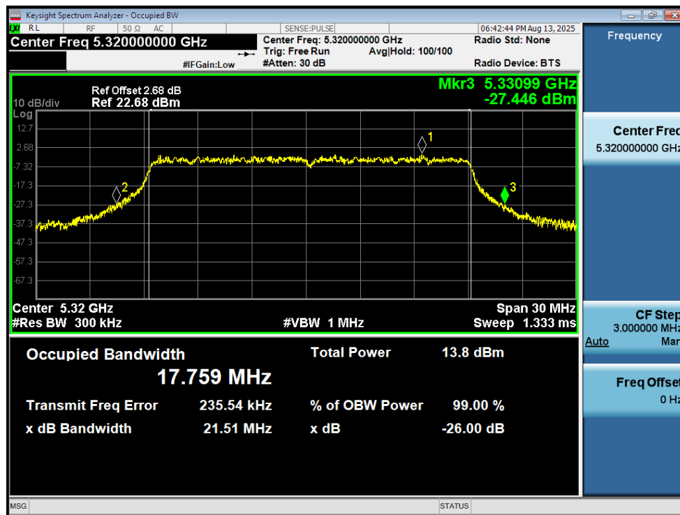
-26dB Bandwidth NVNT n20 5320MHz Ant1
