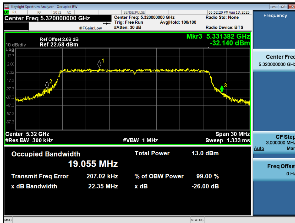
-26dB Bandwidth NVNT ax20 5320MHz Ant1
