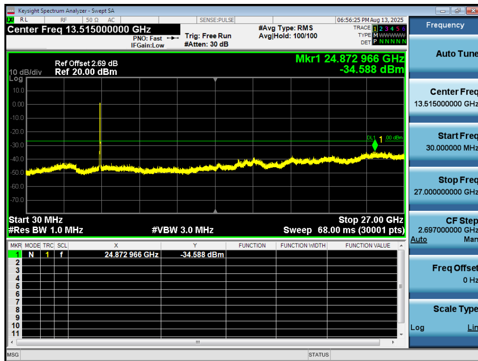
Tx. Spurious NVNT n40 5310MHz Ant1 Emission
