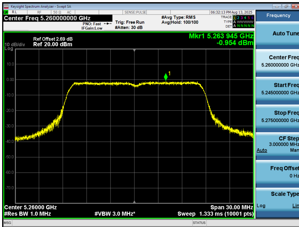
PSD NVNT a 5260MHz Ant1
