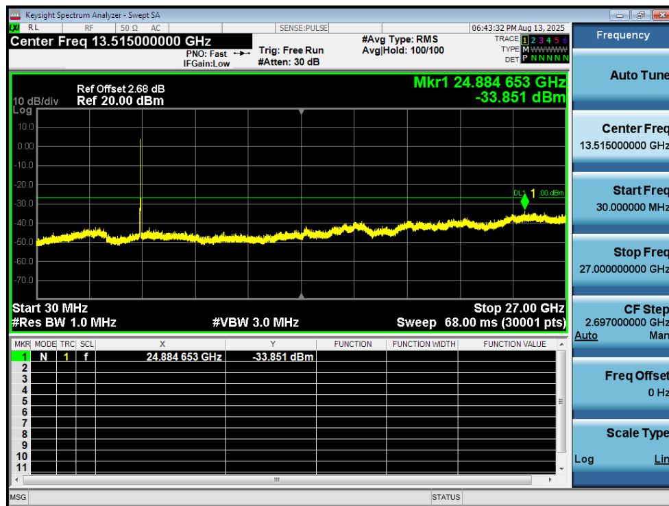
Tx. Spurious NVNT n20 5320MHz Ant1 Emission
