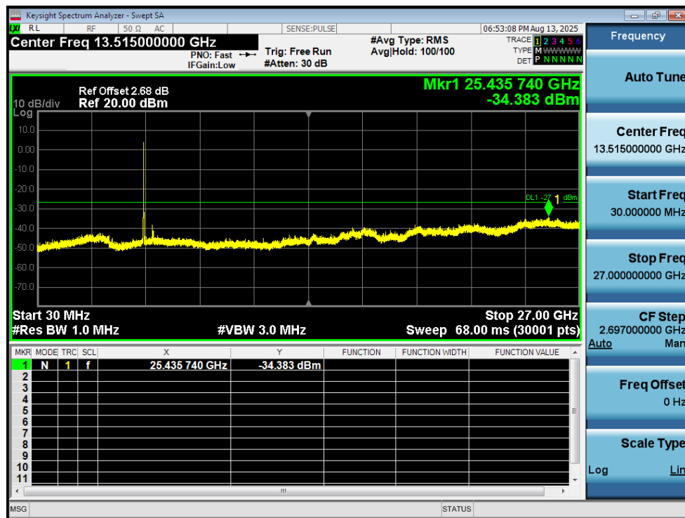
Tx. Spurious NVNT ax20 5320MHz Ant1 Emission
