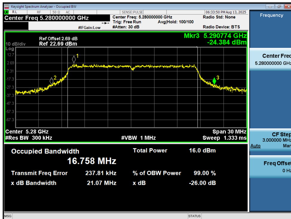
-26dB Bandwidth NVNT a 5280MHz Ant1
