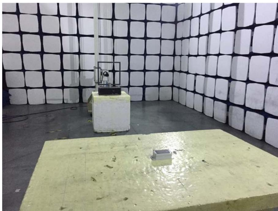
**Radiation Emission Test Setup (30MHz to 1GHz)**
