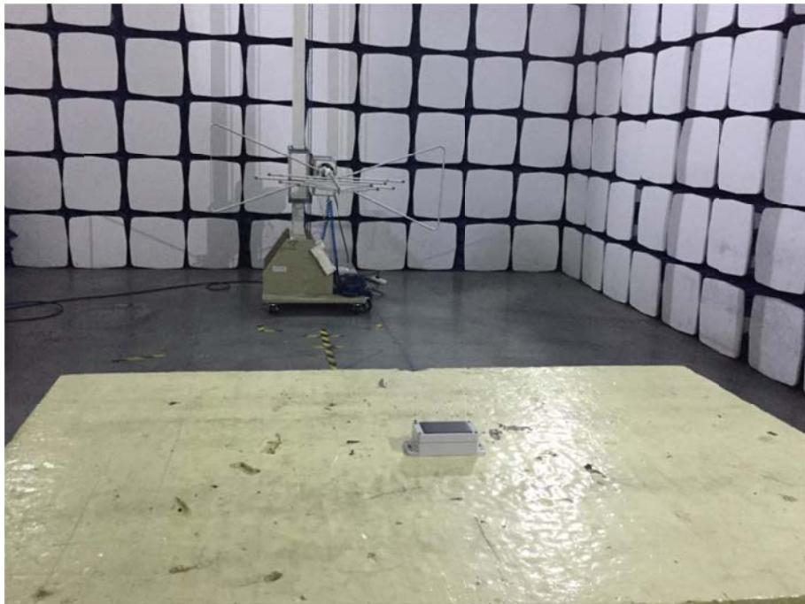
**Radiation Emission Test Setup (Above 1GHz)**
