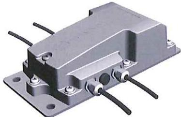
The SAVVY SenseGateway-ExR is a sensor gateway which can connect with an Ex pressure sensor and a maximum of three Ex temperature sensors or Ex switches. The gateway communicates wirelessly with the telematics device SAVVY CargoTrac-ExR according to the IEEE802.15.4 standard, which transmits the measurement data to a portal via the Internet.
