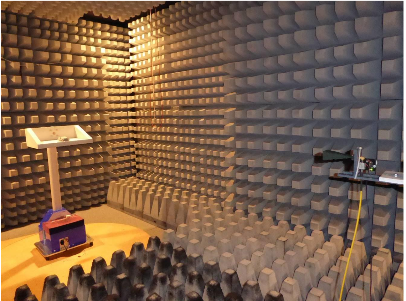
Test setup – radiated test in anechoic chamber Preliminary and final measurement 18 – 26.5 GHz
