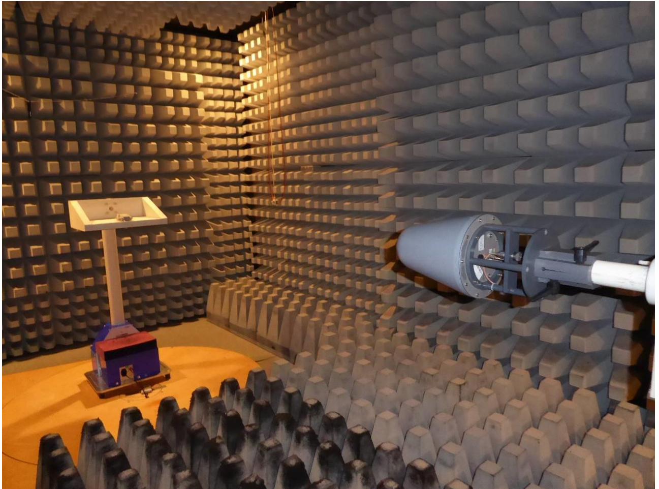
Test setup – radiated test in anechoic chamber Preliminary and final measurement 1 - 12 GHz
