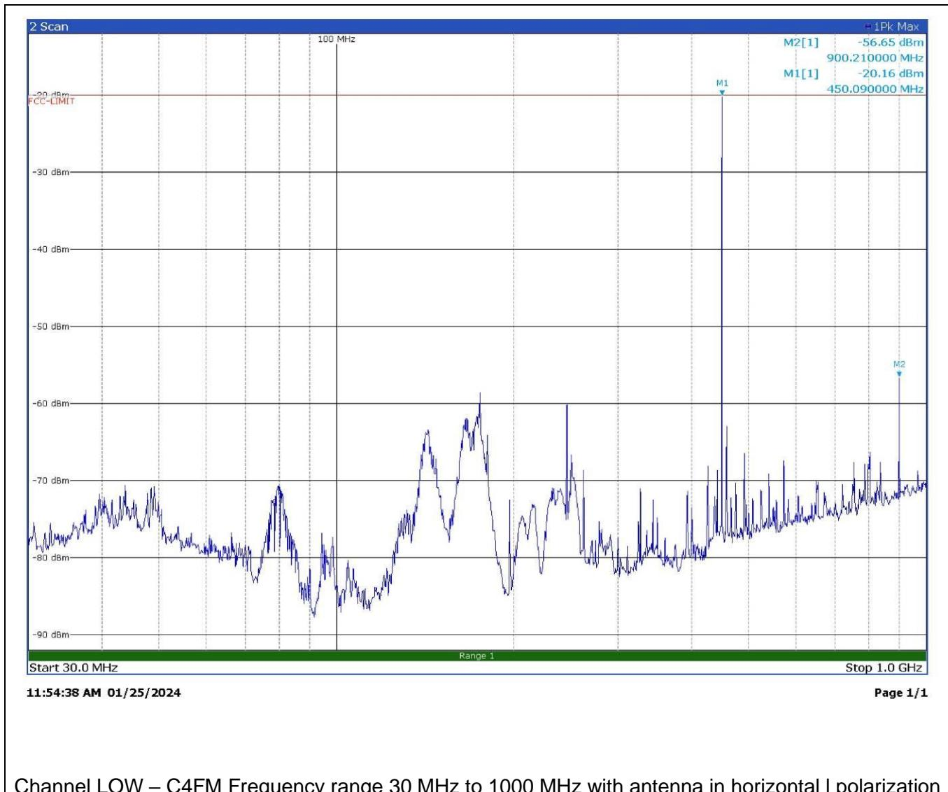
Channel LOW – C4FM Frequency range 30 MHz to 1000 MHz with antenna in horizontal I polarization
