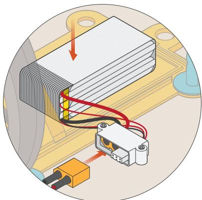
Add back the battery and connect the cables.
