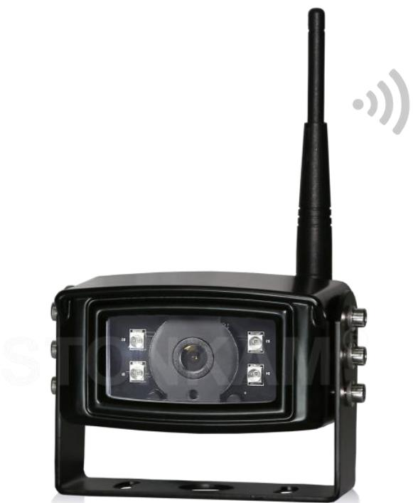
**1080P 2.4GHz Digital Wireless Rear View Camera**
