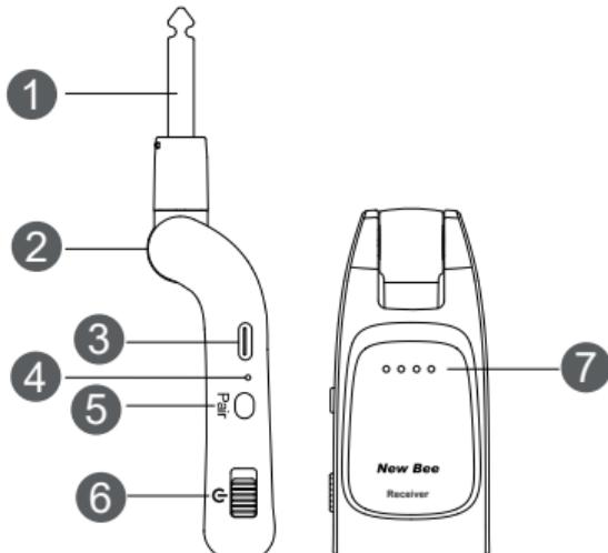
① **Signal-output Plug.** It can be connected to the loudspeaker box or effector.
