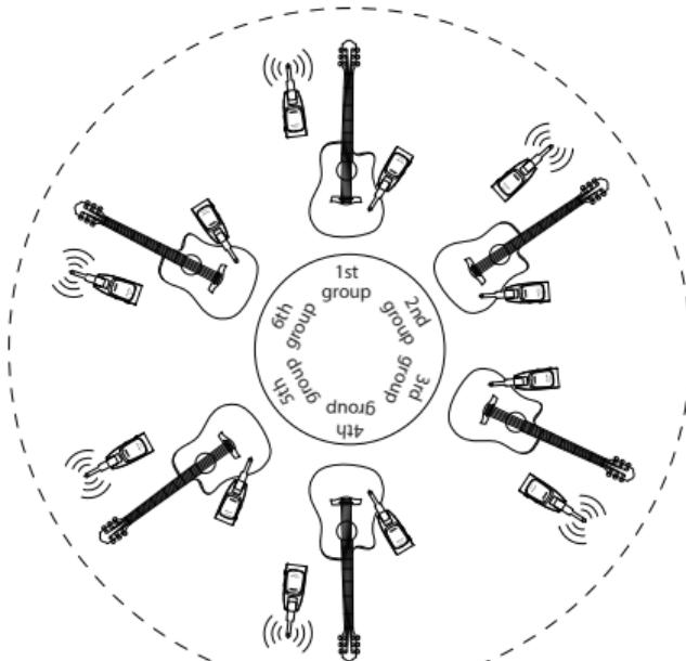
② The wireless system can support one transmitter to send signals to six receivers ( the same product model).
