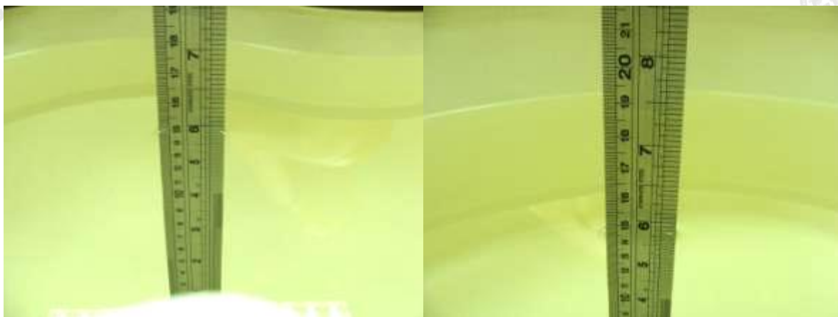
Photo of Liquid Height for Head SAR
