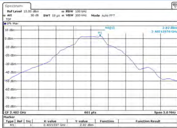
GFSK LOW CHANNEL, CARRIER LEVEL
