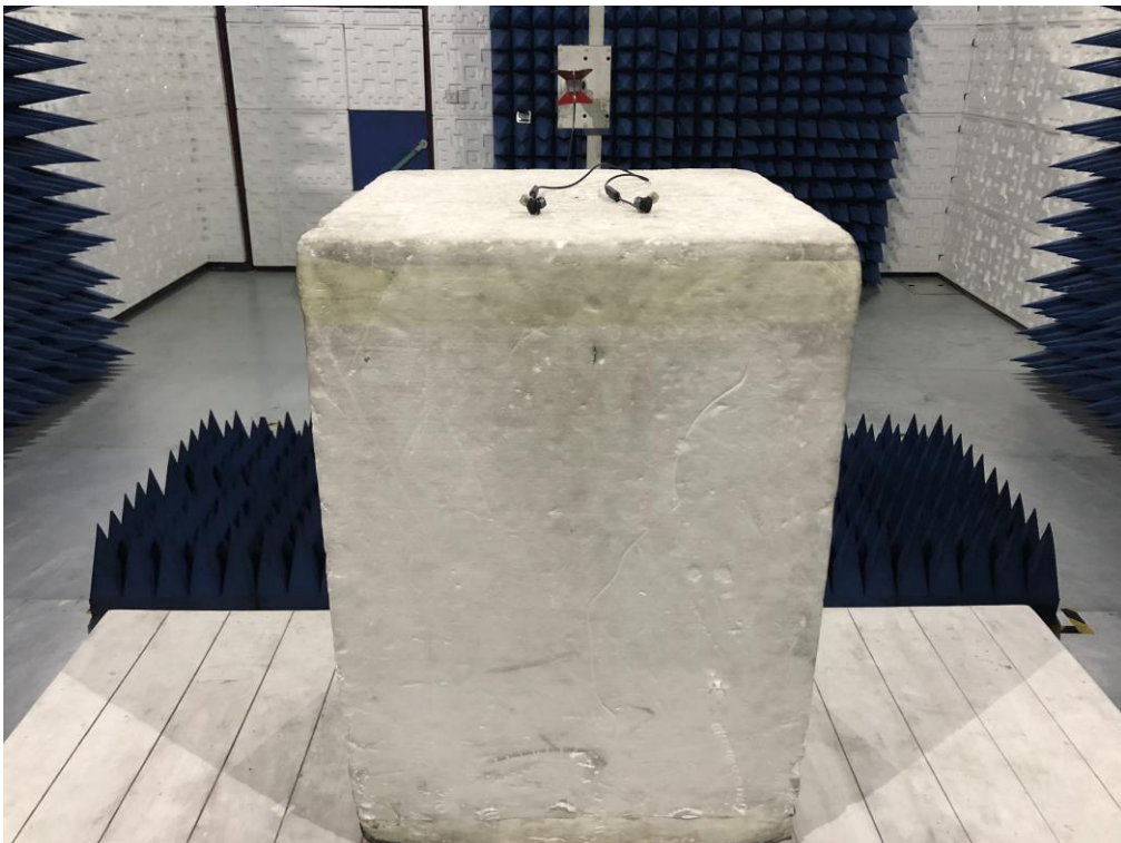
RADIATED EMISSION TEST SETUP ABOVE 1GHZ
