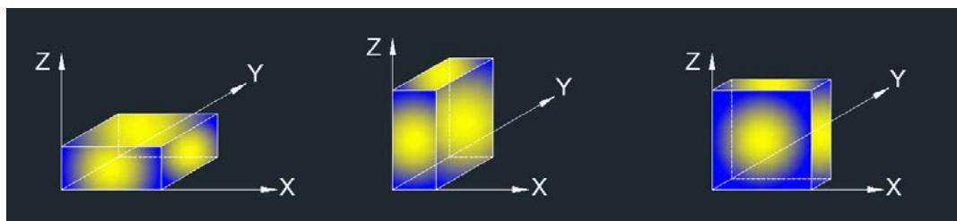
Note 1: For all radiated test, EUT in each of three orthogonal axis emissions had been tested, but only the worst case (Z axis) data recorded in the report.
