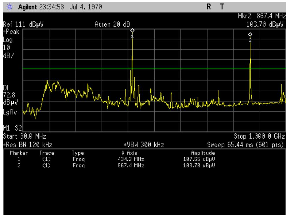
Fundamental peak measurement at 433.9 MHz
