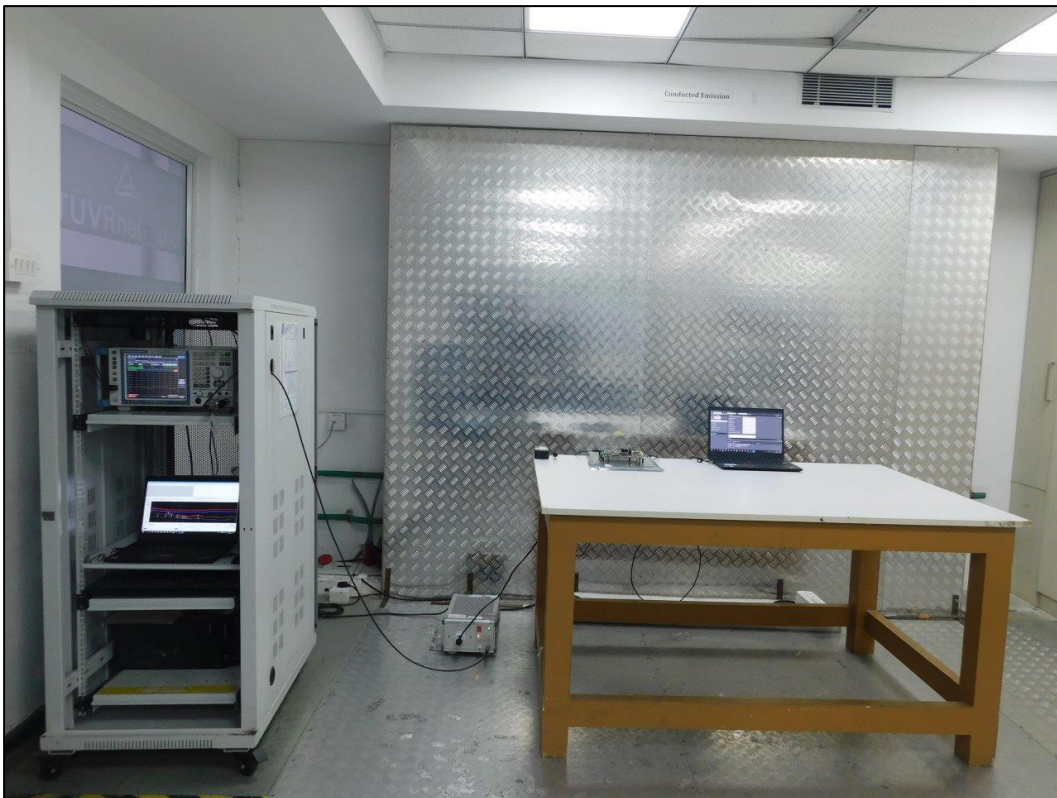
Conducted AC Power line Setup
