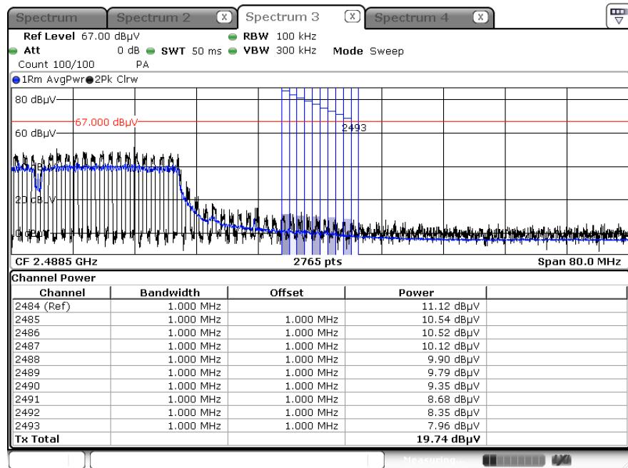
Radiated Restricted Band Edges plot – Peak Result (802.11n (HT40) , MCS0, Ch.9, X-H)
