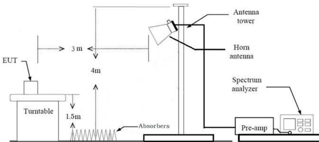
**Test Procedure of Radiated spurious emissions (Below 30 MHz)**
