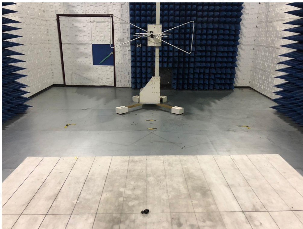
RADIATED EMISSION TEST SETUP ABOVE 1GHZ
