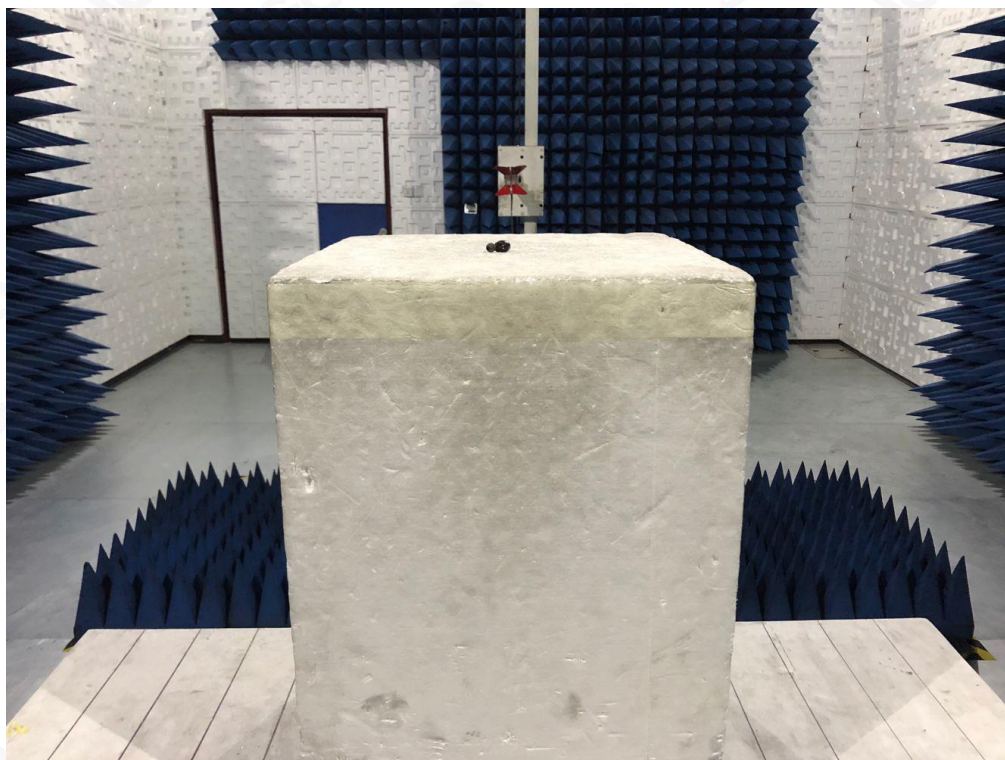
RADIATED EMISSION TEST SETUP ABOVE 1GHZ
