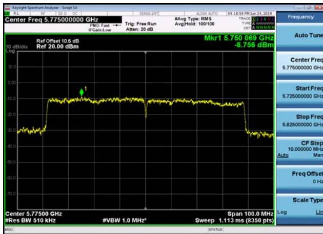
U-NII-3 Power spectral density-802.11 ac(80MHz),5775MHz,Ant1
