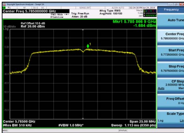
U-NII-3 Power spectral density-802.11 n(20MHz),5825MHz,Ant1
