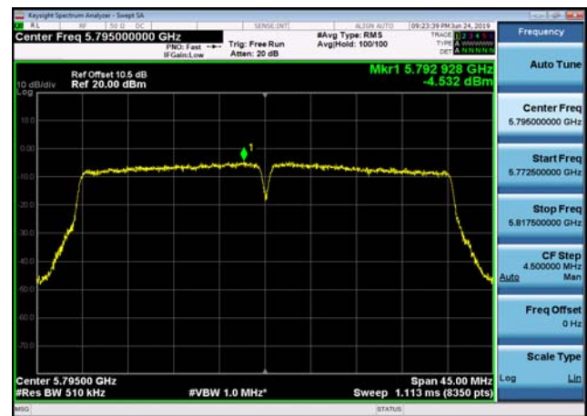
U-NII-3 Power spectral density-802.11 ac(40MHz),5795MHz,Ant2
