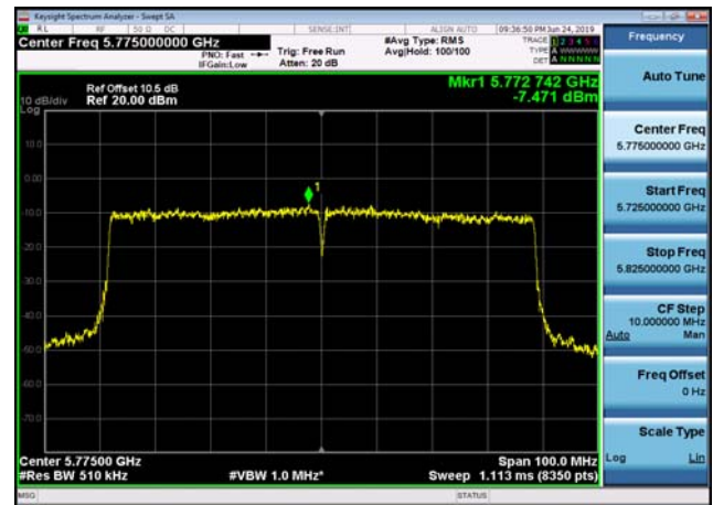
U-NII-3 Power spectral density-802.11 ac(80MHz),5775MHz,Ant2
