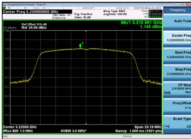
U-NII-1 Power spectral density-802.11 ac(20MHz),5240MHz,Ant1
