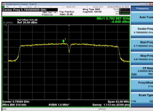
U-NII-3 Power spectral density-802.11 ac(40MHz),5795MHz,Ant1
