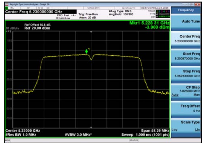
U-NII-1 Power spectral density-802.11 a(20MHz),5180MHz,Ant2
