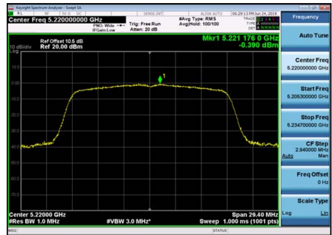
U-NII-1 Power spectral density-802.11 ac(20MHz),5240MHz,Ant2
