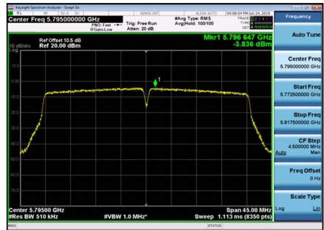
U-NII-3 Power spectral density-802.11 a(20MHz),5745MHz,Ant2
