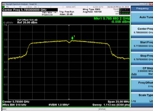
U-NII-3 Power spectral density-802.11 a(20MHz),5785MHz,Ant1
