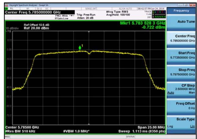
U-NII-3 Power spectral density-802.11 ac(20MHz),5785MHz,Ant2
