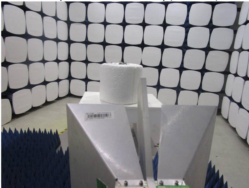
Remark: the PCB with RF eletrical part was tested in 1.5m in rotatable table as worse case mode instead of completed sample.
