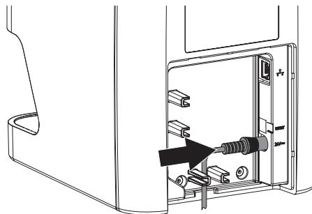
› Plug the mains plug into the power outlet.
