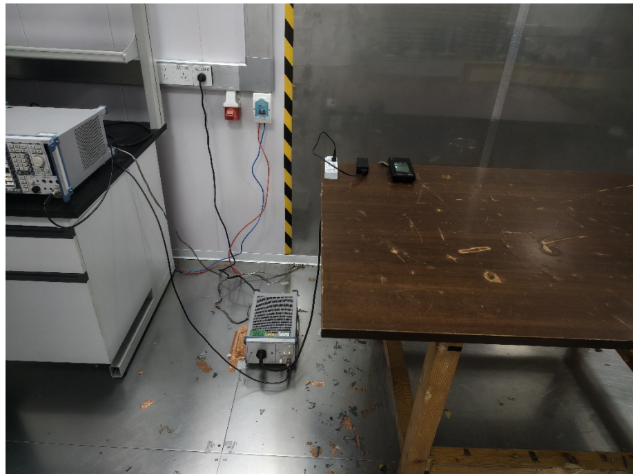
Conducted Emission Test Setup
