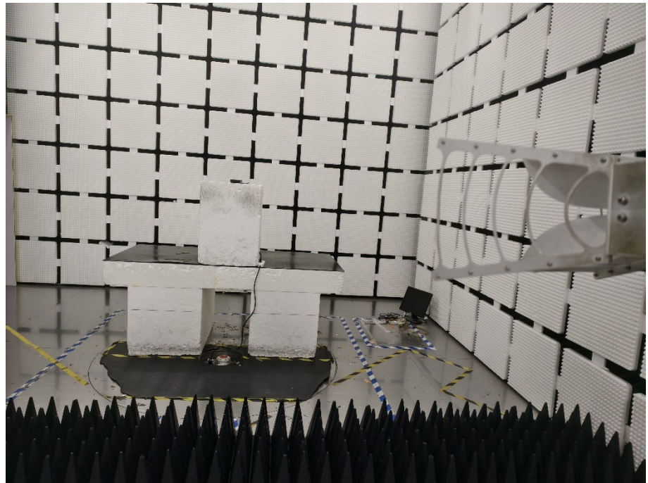
Radiation Emission Test Setup (1GHz to 18GHz)
