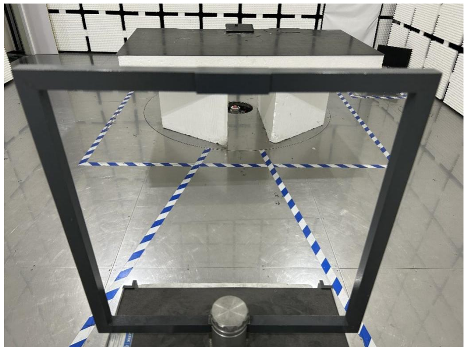
Radiation Emission Test Setup (Below 30MHz)
