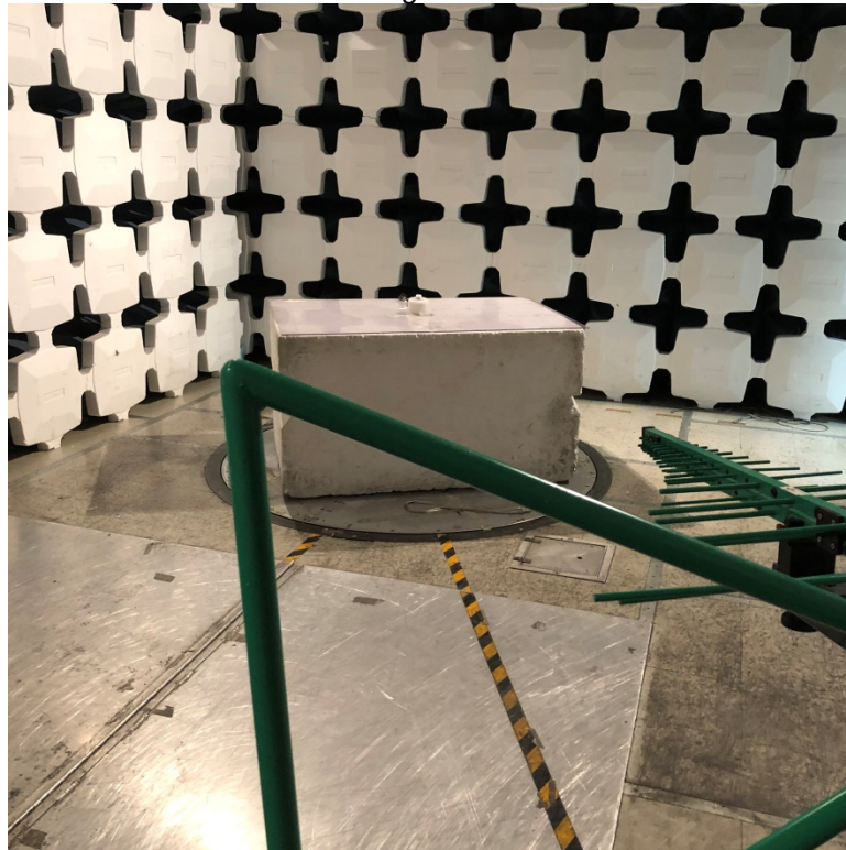
Test Setup for Spurious Radiated Emissions – 30MHz to 1GHz, Horizontal Polarization
