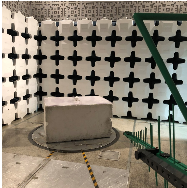
Test Setup for Spurious Radiated Emissions – 30MHz to 1GHz, Vertical Polarization
