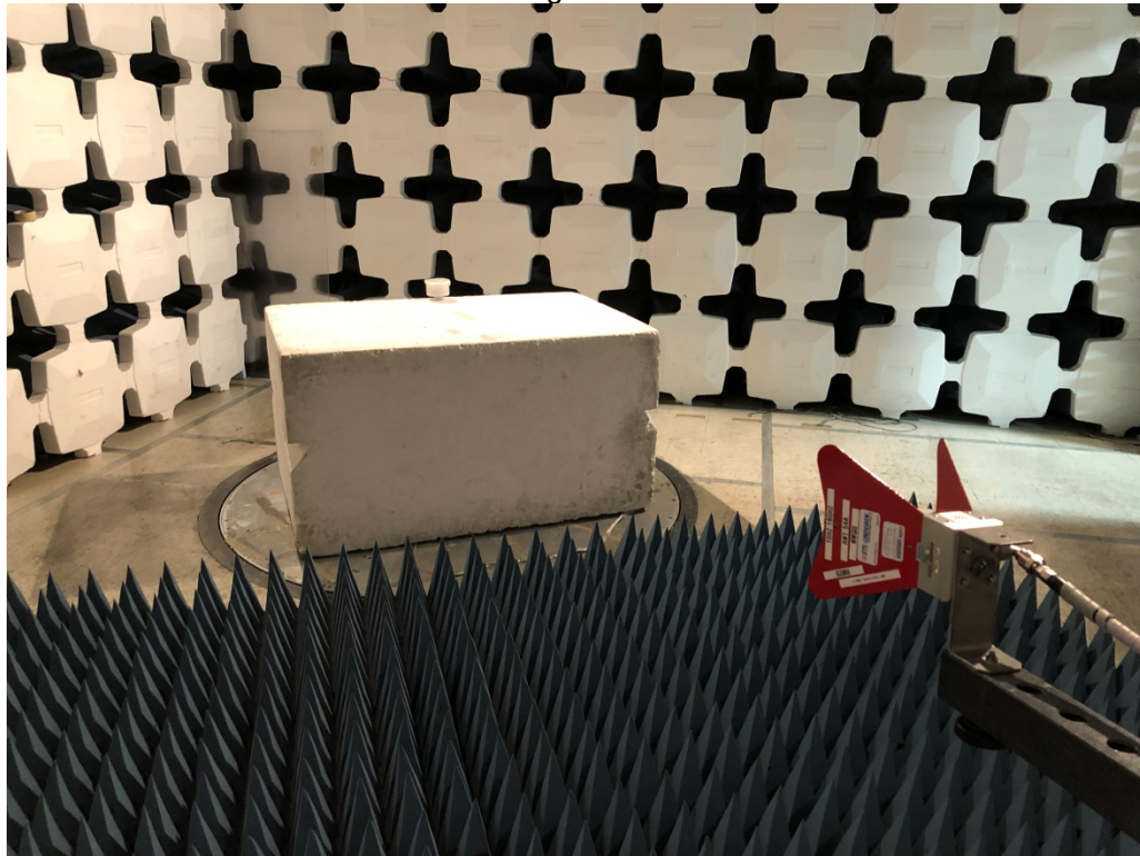
Test Setup for Radiated Emissions – 1GHz to 12.5GHz, Horizontal Polarization
