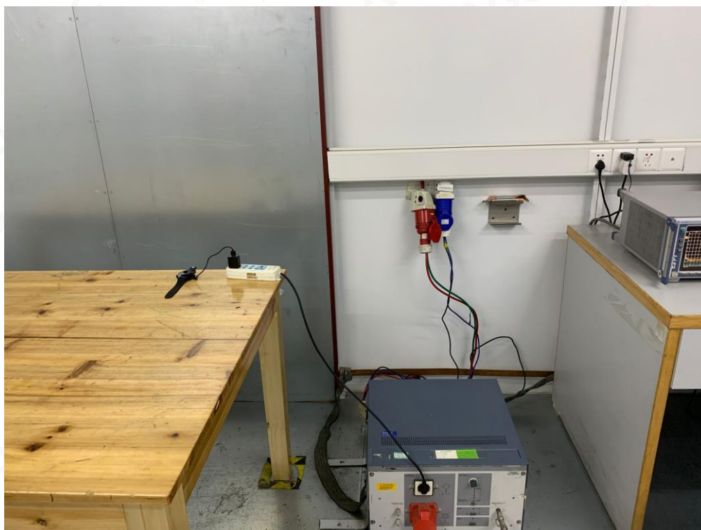
RADIATED EMISSION TEST SETUP BELOW 1GHZ
