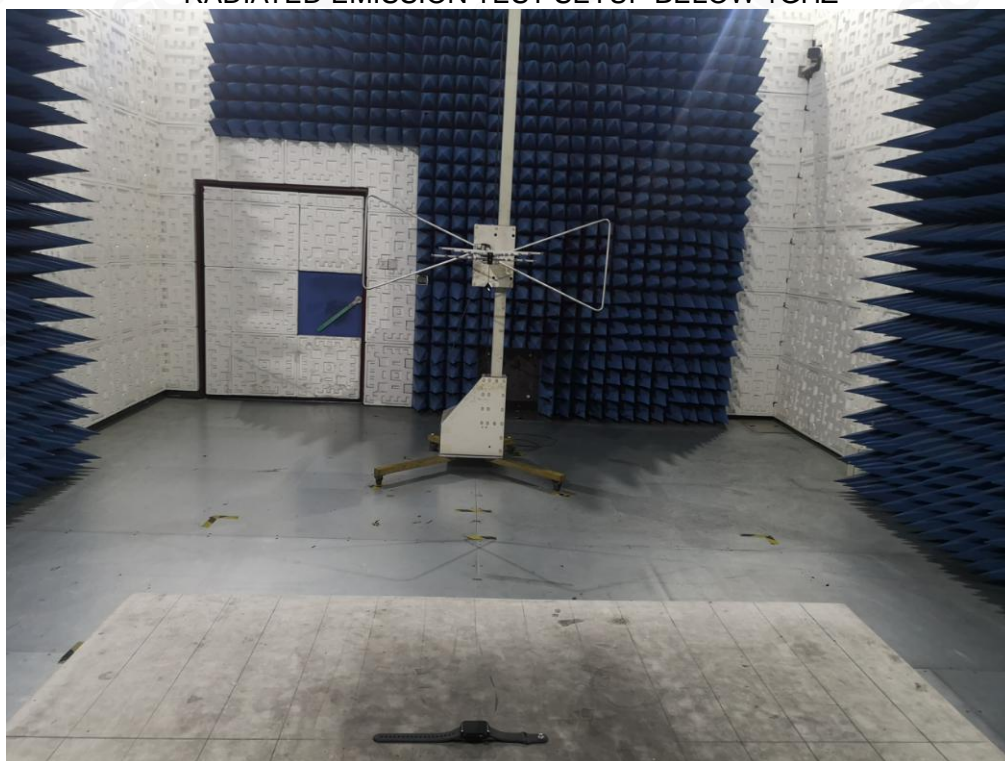
RADIATED EMISSION TEST SETUP BELOW 1GHZ
