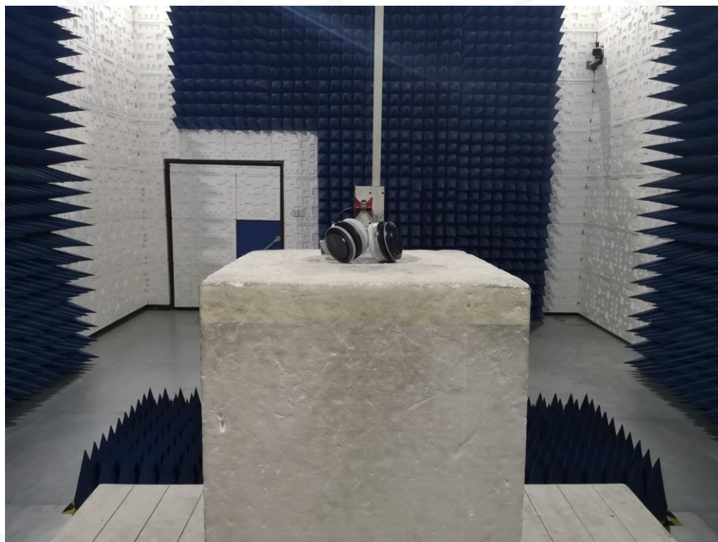
RADIATED EMISSION TEST SETUP ABOVE 1GHZ
