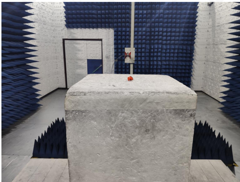
RADIATED EMISSION TEST SETUP ABOVE 1GHZ
