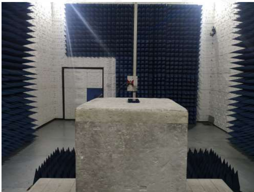
RADIATED EMISSION TEST SETUP ABOVE 1GHZ
