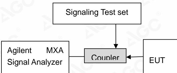
**Test Instrument & Measurement Setup**
